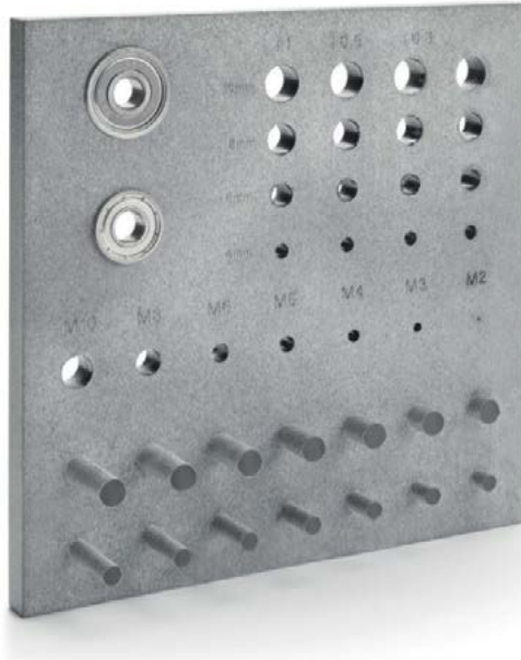
Figure 3: Bearings inserted into an HP MJF part
